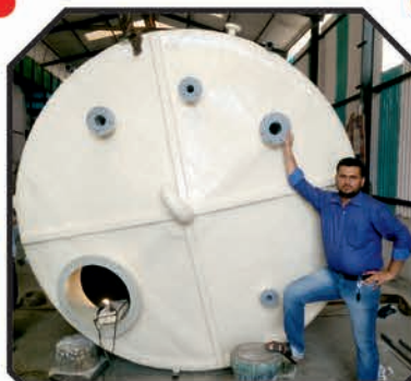
PPGL FRP STORAGE TANK 20KL
